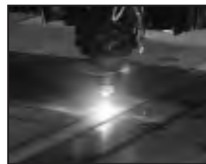
CO 2 laser welding of carbon steel to stainless.
